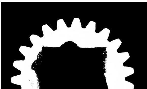
Fig. 3. Acquired image after Thresholding
