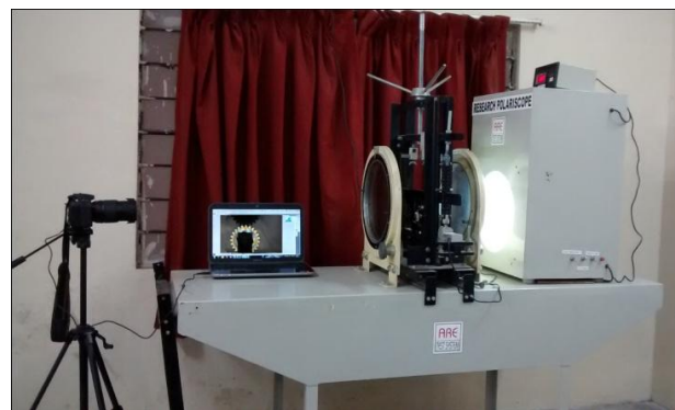
Fig. 1. A simple Machine Vision System.
